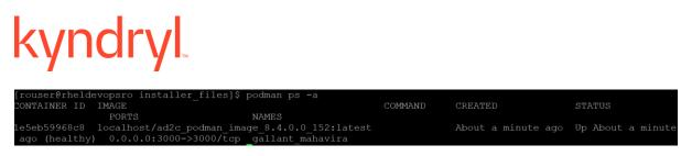
6. Ensure the container should be up and running in healthy state. Now go to the installation directory path specified in the property file. Ensure that the source and output folders are available. The contents of the source/data directory are to be treated as sample data. Replace the contents with the actual data applicable to your environment and your requirements.
