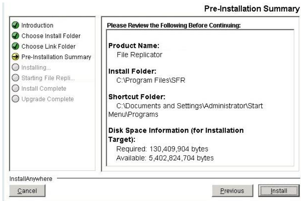
Figure 13. Upgrading File Replicator - Preinstallation Summary
